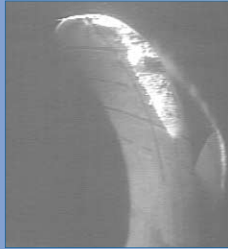
A vapour cavity forms along a propeller blade. As vapour cavities form and collapse, cavitation noise occurs.
