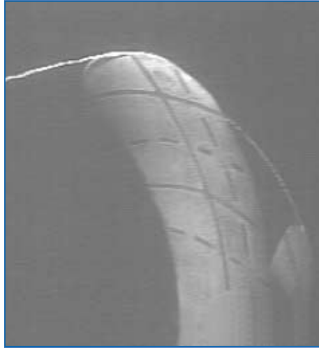
A vapour cavity forms along a propeller blade. As vapour cavities form and collapse, cavitation noise occurs.
